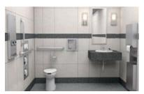
"Parry Ware" sanitary fittings floor mounted EWC & Washbasin and "JAGUAR florentine" C.P. fitting, wall dado up to 7'0" height, 12" x 12" anti-skid tiles as flooring, P.V.C pipes for outer plumbing lines and CPVC pipes for concealed water line and Geyser provision, water proof vinyl coated flush door, UPVC ventilators with exhaust fan provision and MS grill.
